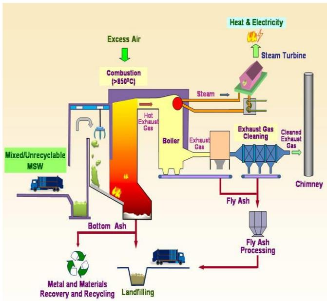
Fig.2- Waste-to-energy incinerator with pollution controls that burns mixed solid waste [17].
