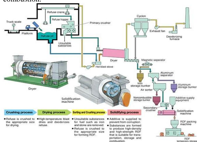
Figure 5. Refuse Derived Fuel Plant [22].
