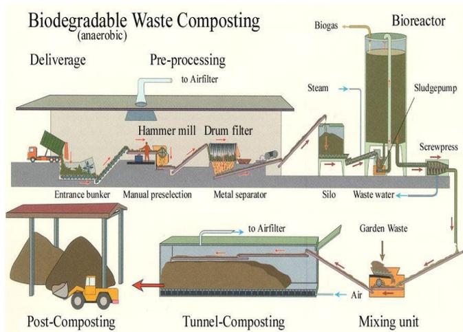
Figure 4. Anaerobic Composting [21].
