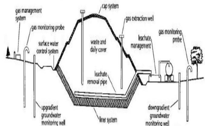
Fig.1- A typical Sanitary landfill [11].
